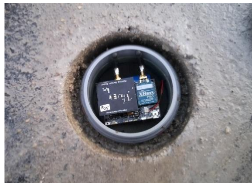
Wireless vehicle-presence sensor with 7 to 10 years of battery life
